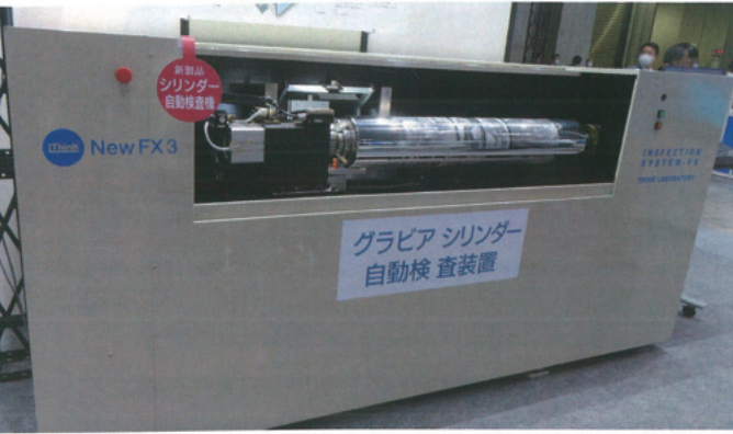
This is the standard equipment on the New FX3, and the surface inspection of cylinders is fully automated
